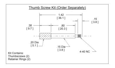
Note: The  $3M^{\text{TM}}$  3341-7 Thumb Screw contains lead in the base material, therefore RIA E5 & C3 apply when using this hardware.
